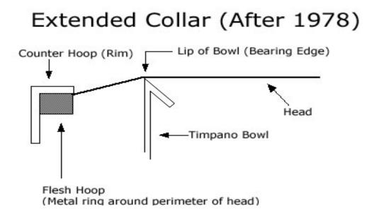
The best way to determine the correct size head you need is to take the head off the drum and measure the outside diameter of the head. Outside diameter means from one side of the metal ring to the other. If the head is still on the drum, you can measure from inside one tension rod across to the opposite tension rod:
